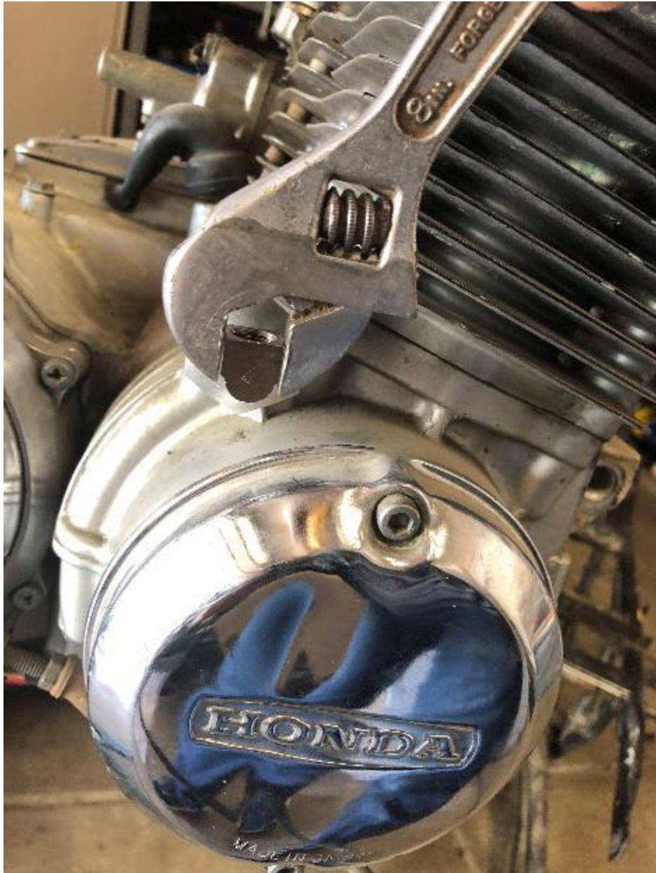
Figure 6 Tighten hand tight plus 1-2 turns, until snug
